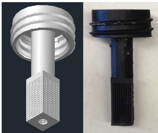
Figure 8 CI Porous Box. Left – CAD drawing. Right – 3D printed CI
